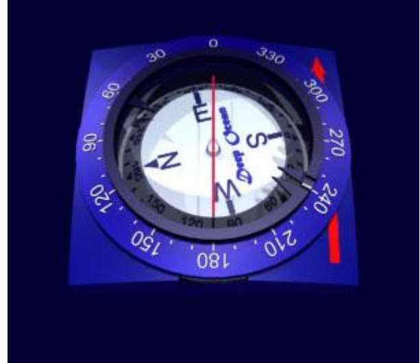
Rotate the bezel such that the double markers points to 240 degrees.
