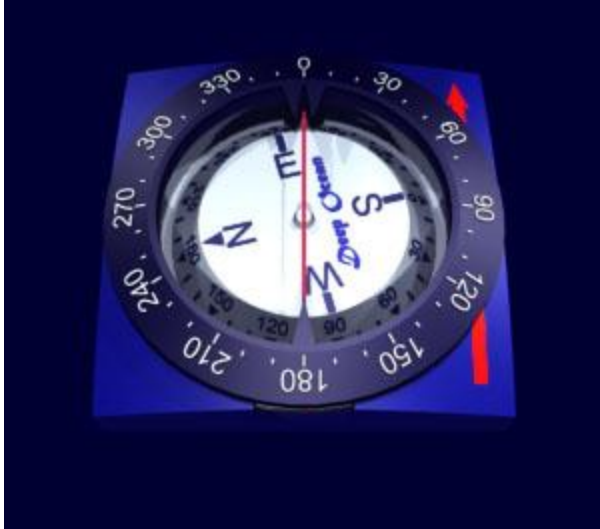
Indirect reading compass: starting position. The magnetic card points to the North, the bezel is in the default position.
