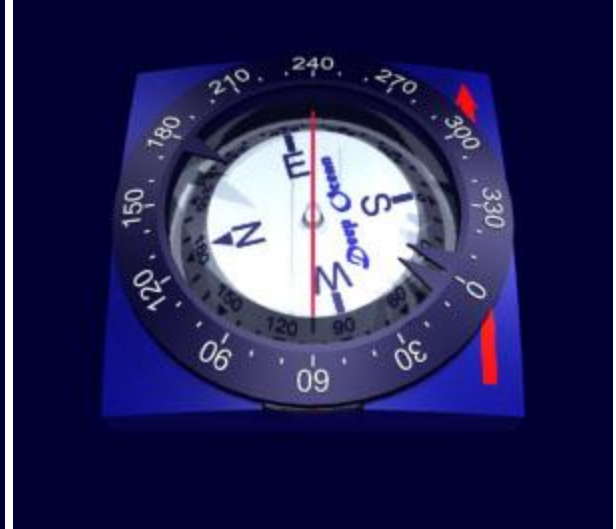
Rotate bezel until the 240 degrees mark on it corresponds to the lubber line.
