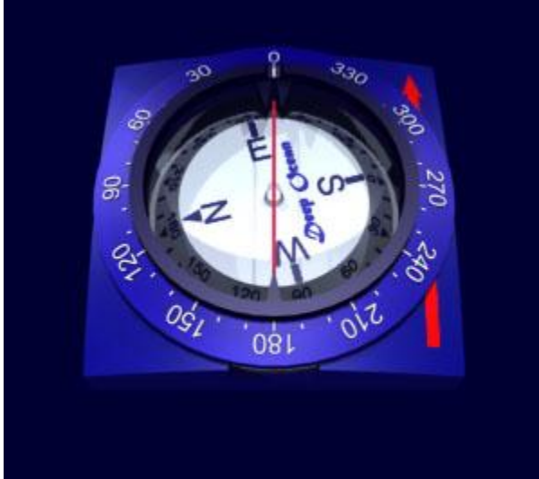
Direct reading compass: starting position. The magnetic card points to the North, the bezel is in the default position.
