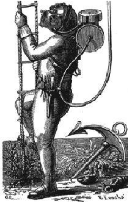
Figure 3. Aerophore patented in 1865 by Benoit Et Rouquayrol and Auguste Denayrouse. (Courtesy Historical Diving Society)
